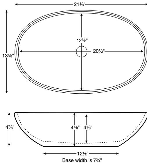
NOTE: Sink rests on top of counter. Cut-out for the drain installation is required. Measurements are  $\pm 1/2$ " and are subject to change without notice. Data herein supersedes all previous prior to publication date indicated below.
