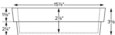
NOTES: SINK IS SEMI-RECESSED. SINK MUST BE MEASURED ON-SITE TO ENSURE ACCURATE DIMENSIONS OF HOLE CUT-OUT. Measurements are  $\pm 1/2$ " and are subject to change without notice. Data herein supersedes all previous prior to publication date indicated below.
