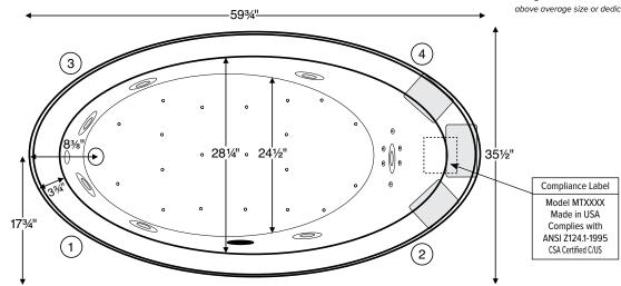
$\label{lem:numbered} \mbox{Numbered areas outside of tub represent possible stub-out locations for cleaning systems and Breda valves.}$
