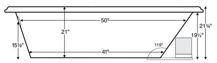
IMPORTANT: Air baths and tubs with a pre-leveled foam base add 2-3" to overall tub height.
