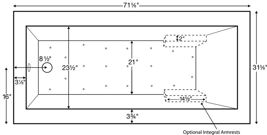
The Sculpted Finish process does not allow enough space for mounting fixtures on the tub deck.
